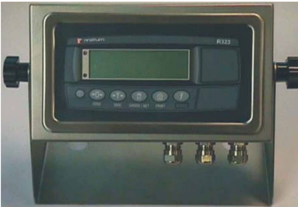
Figure 2 - Rinstrum Model R323 Indicator Module in a Rinstrum Housing
