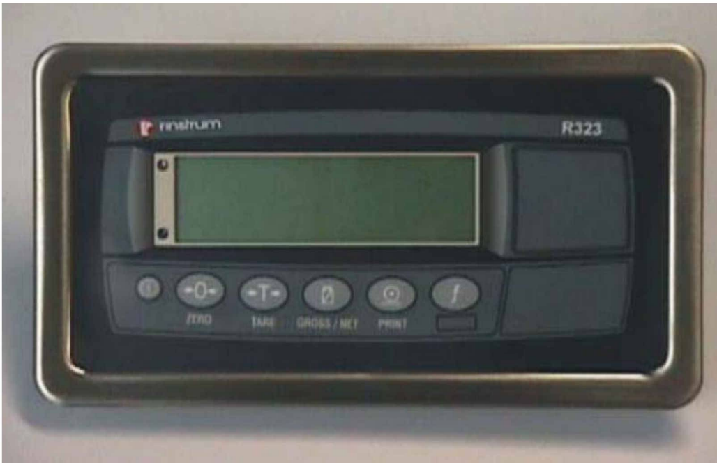
Figure 2 - Rinstrum Model R323 Indicator Module in a Rinstrum Housing
