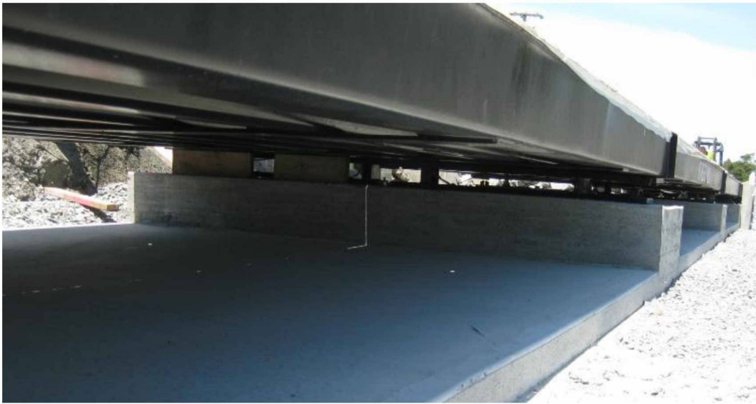
Figure 1.2 - Above Ground (pit-less type) installation
